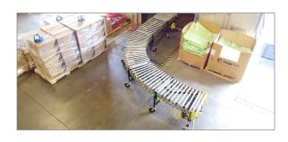
Unsatisfied with powered flexible conveyors on the market, CASI built its own. CASI's powered conveyor is the perfect solution. It's Americanmade and is high quality with better lead-times and lower pricing.
